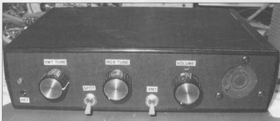
Figure 7—The completed transceiver, installed in a “not so ugly” enclosure.
